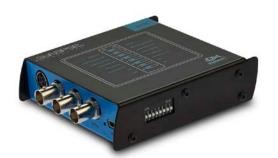
"Vizrt is pleased to qualify and recommend the Bluefish444 Synapse converters because they are reliable and tailored to broadcasters needs," said Gerhard Lang, Chief Engineering Officer at Vizrt. Features like a redundancy input channel, support for 3G SDI & HDMI conversion, audio muxing, downscaling and SDI preview ensure that Synapse converters are highly suitable for the majority of Vizrt's customers."
